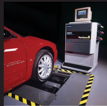
An ASM Analyzer can tell if a car has acceptable levels of emissions. Car emissions directly effect the environment.
